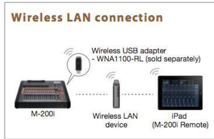
Using a Wireless USB adapter, connect the M-200i to a wireless LAN device such as a router to establish a wireless connection with an iPad.
