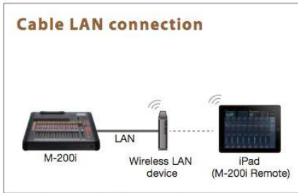
Connect the M-200i with a Cat5e/6 cable to a wireless LAN device such as a router to establish a wireless connection with an iPad.
