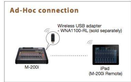
Connect the M-200i directly to an iPad without using wireless devices such as a router.
